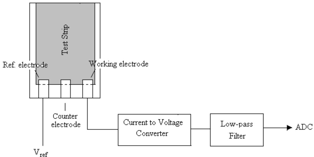
**Figure 6:** A schematic diagram of the glucose test strip and glucose detection unit meter [5]
