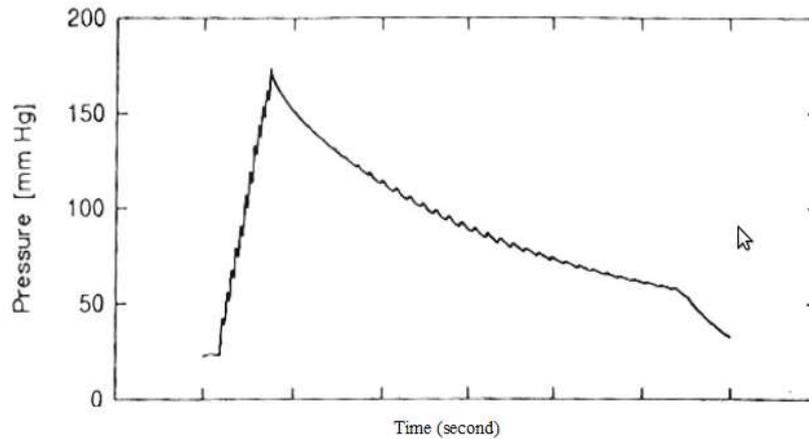
**Figure 1:** A recording of cuff pressure. The pressure is initially raised rapidly and then lowered slowly [4].
