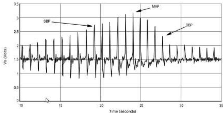
**Figure 4:** Extracted oscillation signal at the output of the amplifier [3].
