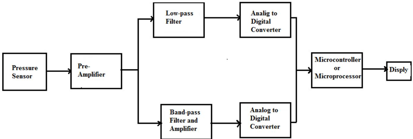
Figure 2: Block diagram of the device [2].
