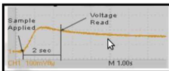
**Figure 7:** Glucose voltage curve [6]
