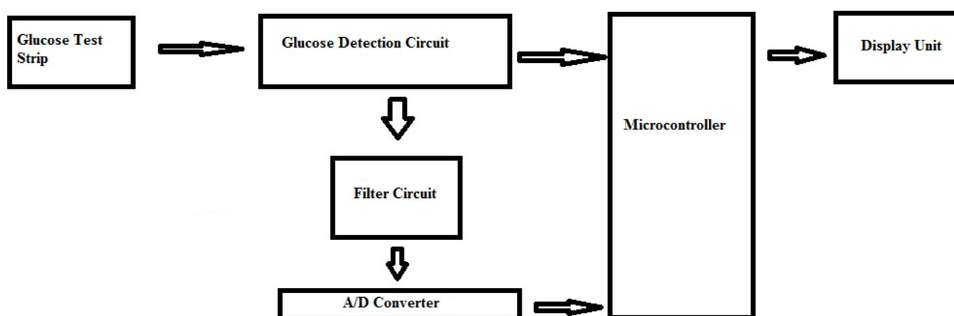
Figure 5: Block diagram of Glucose meter [6].
