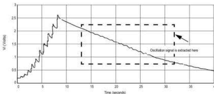
**Figure 3:** Cuff pressure signal at the output of the pressure sensor [3]
